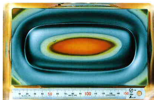
Fig. 10 The optical photograph of the surface of the ultra high density target at the end of its life.
