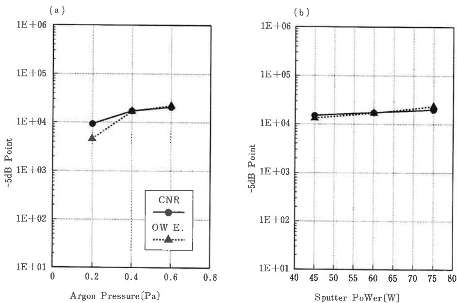
**Fig. 17** Dependences of  $-5\text{dB}$  point on sputter conditions of active layer. (a)  $-5\text{dB}$  point as a function of Ar pressure. (b)  $-5\text{dB}$  point as a function of sputter power. ● and ▲ denote  $-5\text{dB}$  point of CNR change and that of overwrite erasability, respectively.
