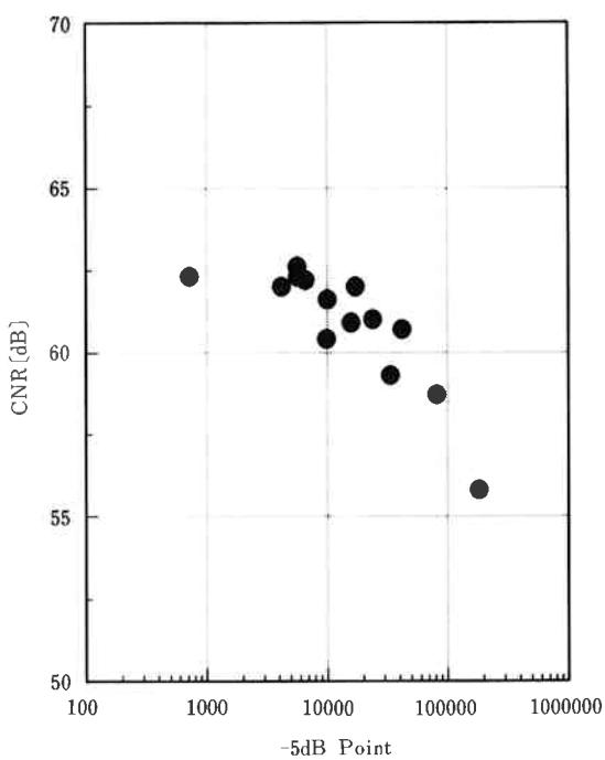
Fig. 15 Relationship between CNR and  $-5\text{dB}$  point of CNR change.
