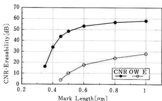
Fig. 22 Dependences of CNR and overwrite erasability on mark length. Sample is made and tuned by conditions for 680nm laser. Data is obtained by 680nm laser, objective lens with NA of 0.55, and linear velocity of 8m/s.
