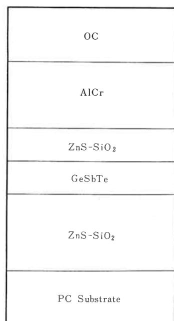
Fig. 4 Cross sectional view of phase change recording disk used in this study.
