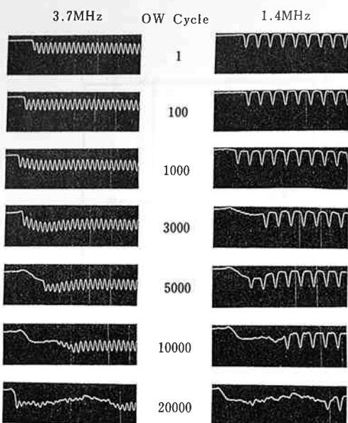
Fig. 20 Playback signal waveforms of 3.7MHz signal (1.5T signal) and 1.4MHz signal (4T signal) in each overwrite cycle number for disk sample made by standard sputter condition.
