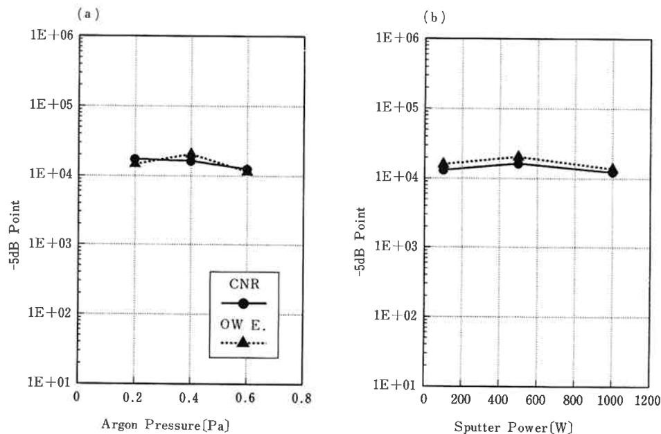
Fig. 19 Dependences of  $-5\text{dB}$  point on sputter conditions of reflective layer. (a)  $-5\text{dB}$  point as a function of Ar pressure. (b)  $-5\text{dB}$  point as a function of sputter power. ● and ▲ denote  $-5\text{dB}$  point of CNR change and that of overwrite erasability, respectively.
