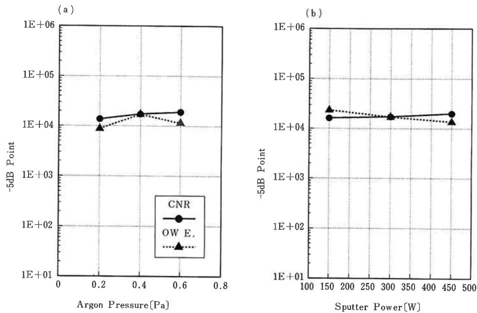
Fig. 18 Dependences of  $-5\text{dB}$  point on sputter conditions of second protective layer. (a)  $-5\text{dB}$  point as a function of Ar pressure. (b)  $-5\text{dB}$  point as a function of sputter power. ● and ▲ denote  $-5\text{dB}$  point of CNR change and that of overwrite erasability, respectively.
