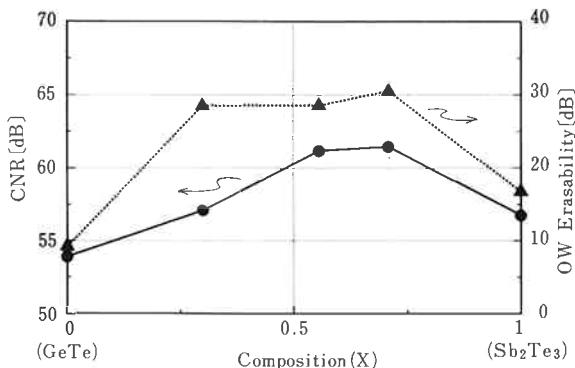
Fig. 10 Dependences of CNR (●) and overwrite erasability (▲) on composition (x) of active layer.
