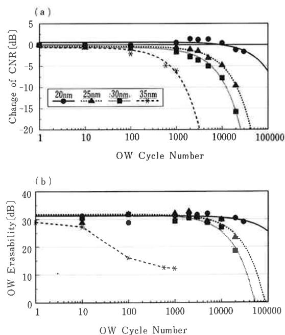
Fig.13 Overwrite cycle characteristics of disk samples with various thickness second protective layer. (a) Change of CNR as a function of overwrite cycle number. (b) Overwrite erasability as a function of overwrite cycle number. ●, ▲, ■ and \* denote 20nm, 25nm, 30nm and 35nm, respectively.
