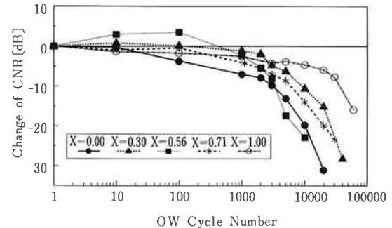
Fig. 11 Change of CNR as a function of overwrite cycle number for disk samples with active layer of various composition. Vertical axis indicates a CNR change from initial value.
