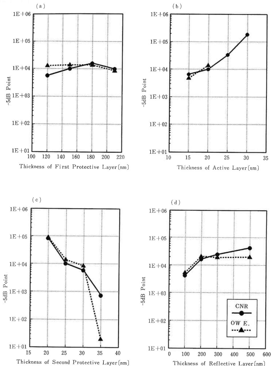
Fig.14 Dependence of  $-5\text{dB}$  point on thickness of each component layer. (a) Dependence on first protective layer. (b) Dependence on active layer. (c) Dependence on second protective layer. (d) Dependence on reflective layer. ● and ▲ denote  $-5\text{dB}$  point of CNR change and that of overwrite erasability, respectively.
