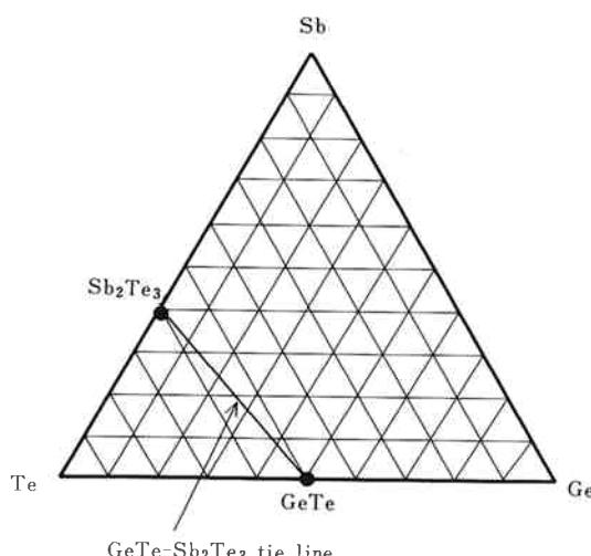
Fig. 3 Triangle composition diagram of GeSbTe system and GeTe-Sb<sub>2</sub>Te<sub>3</sub> tie line.
