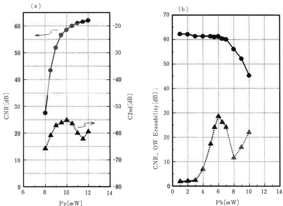
Fig. 9 Recording characteristics of a disk sample with active layer of  $x=0.56$ . (a) Dependences of CNR (●) and second harmonic (▲) as a function of peak power. (b) Dependences of CNR (●) and overwrite erasability (▲) as a function of bias power.
