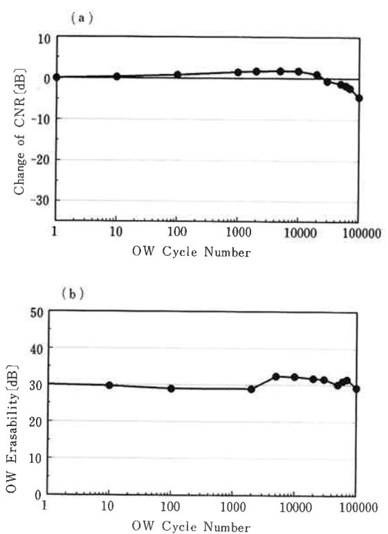
Fig. 21 Overwrite cycle characteristics of disk sample obtained by optimized sputter conditions. (a) Change of CNR as a function of overwrite cycle number. (b) Overwrite erasability as a function of overwrite cycle number.
