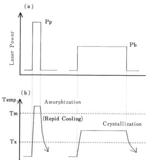
Fig. 1 Laser power patterns (a) and temperature change of active layer (b) for amorphization (recording process) and crystallization (erasing process).
