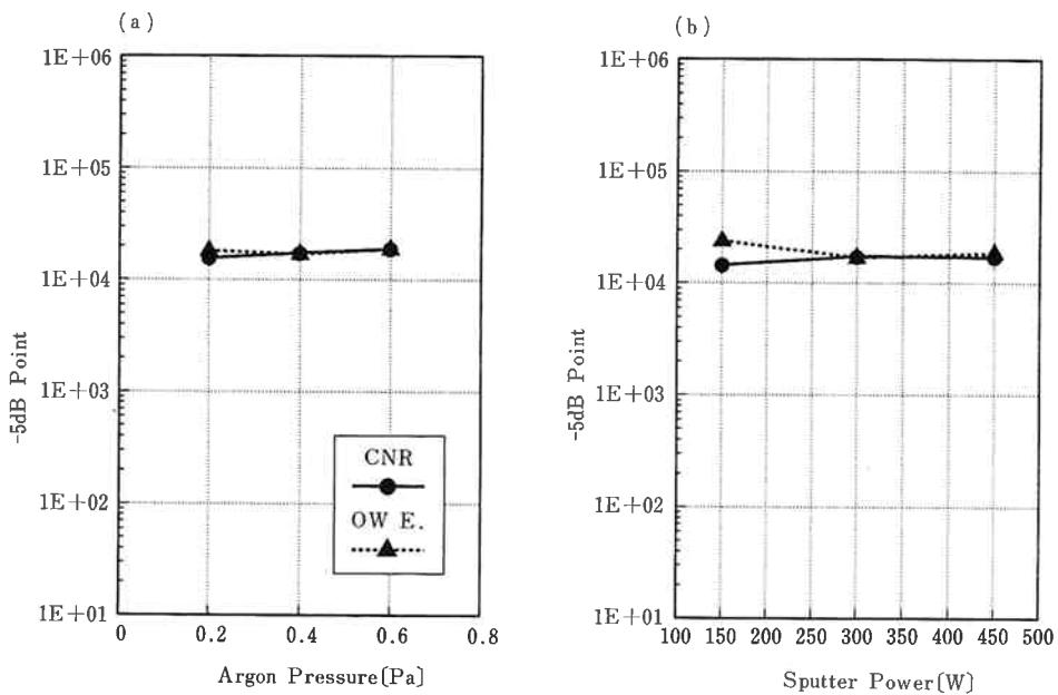
**Fig. 16** Dependences of  $-5\text{dB}$  point on sputter conditions of first protective layer. (a)  $-5\text{dB}$  point as a function of Ar pressure. (b)  $-5\text{dB}$  point as a function of sputter power. ● and ▲ denote  $-5\text{dB}$  point of CNR change and that of overwrite erasability, respectively.
