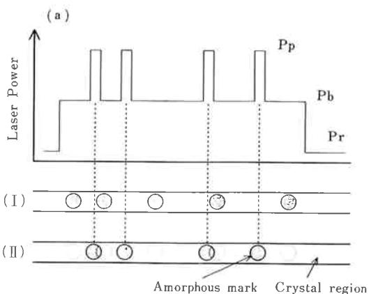
Fig. 2 Concept of 1beam overwrite. (a) Laser power modulation pattern. (I) recording track before overwrite. (II) recording track after overwrite a signal shown in (a). The circles of dotted line in track (II) indicate the erased marks.
