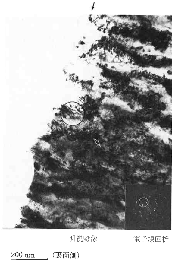
Fig. 11 Bright field image and electron beam diffraction at the back of the stamper
