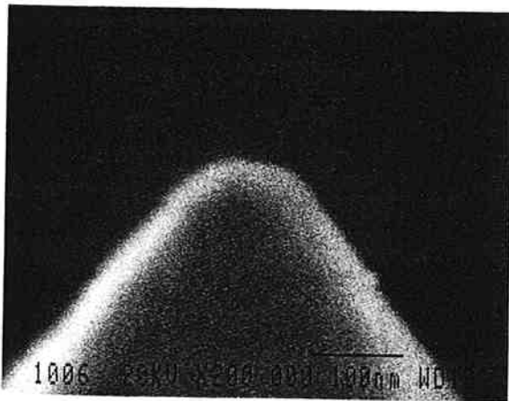
Fig. 4 Tip shape of a conventional AFM probe.
