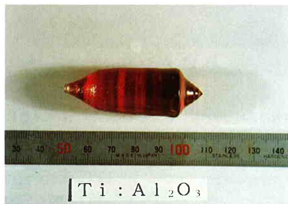
Fig. 2 Bubble free Ti:Al 2 O 3 crystal grown at a pulling rate of 0.4 mm/h and a rotation rate of 50 rpm under He-H 2 atmosphere.
