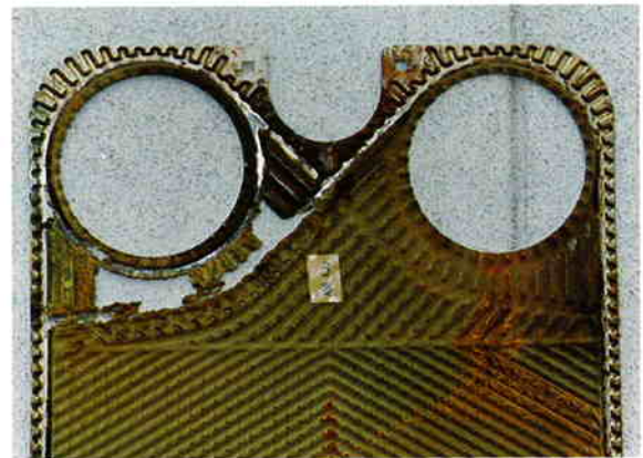
Photo. 3 Appearance of crevice corrosion of titanium
