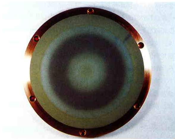
Fig. 12 ITO Target with 85% in Theoretical Density after Sputtering. Total Sputtering Time: 240 min
