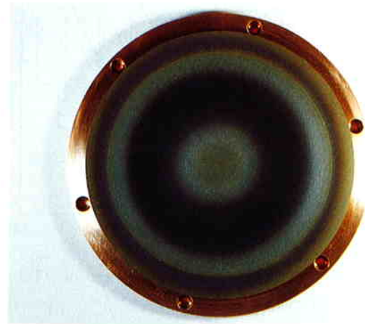
Fig. 13 ITO Target with 67% in Theoretical Density after Sputtering. Total Sputtering Time: 60 min
