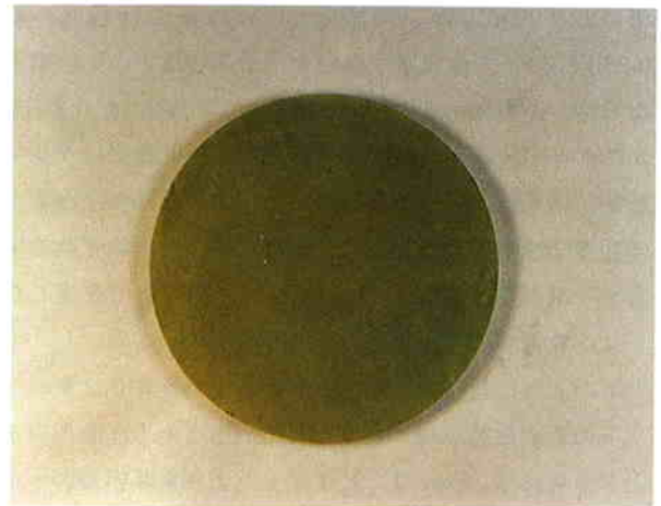
Fig. 15 ITO Target with 67% in Theoretical Density.
