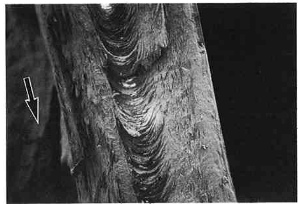
(a) skin layer (quenched) core layer (slow cooled) (×28)
