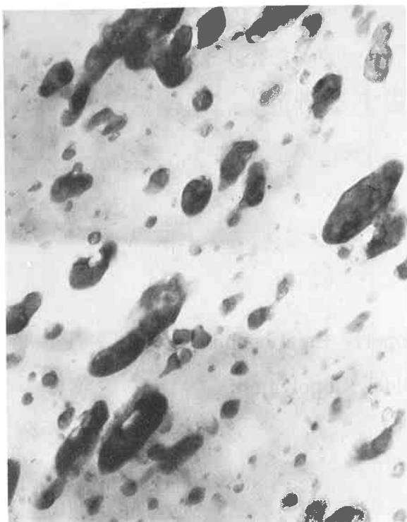
Fig. 1 TEM photomicrograph of an E-P block copolymer
