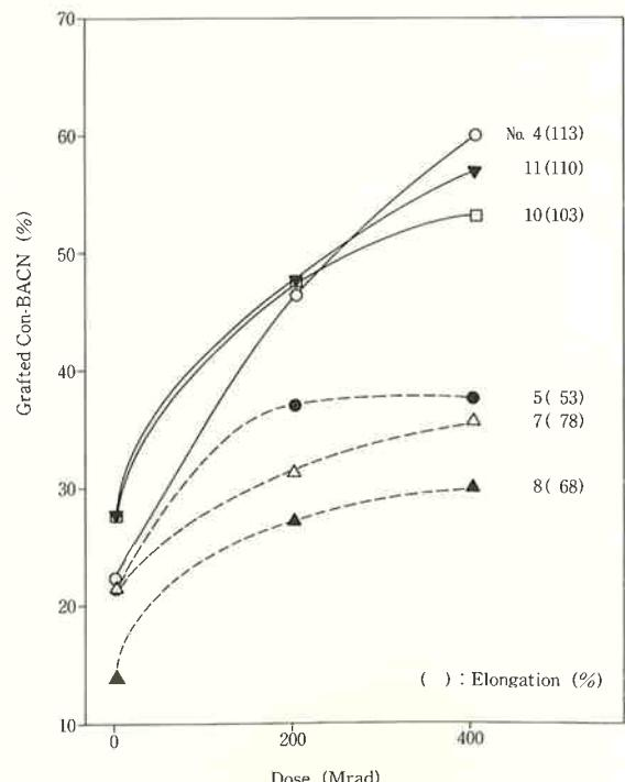
Fig. 9 Change of grafted Con-BACN amount by  $\gamma$ -ray irradiation
