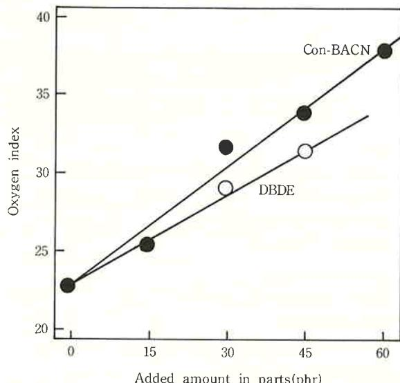
Fig. 11 Oxygen index of EPDM compounds
