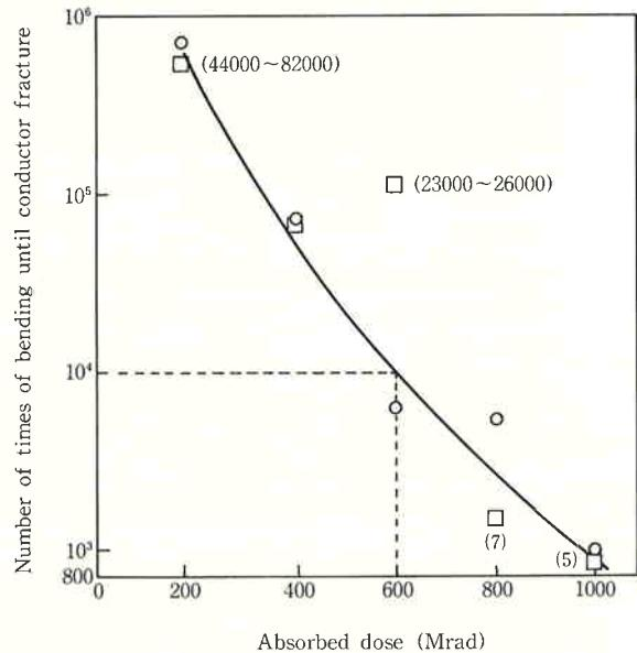
Fig. 13 Radiation resistance of cables in terms of flexibility
