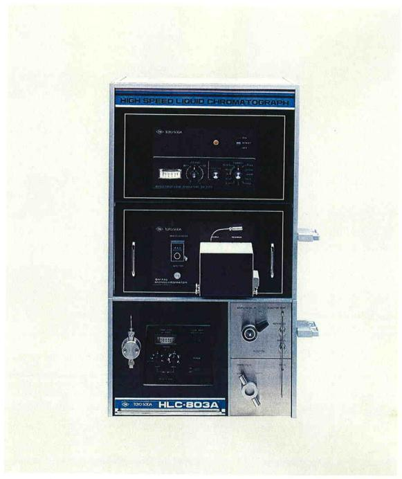
Shown here are high-speed liquid chromatographs HLC-803 A/B newly developed for routine analysis. They feature high performance feed pumps TOYO SODA-ALTEX 110A/100A and work well with every detection system one needs for his purpose.
