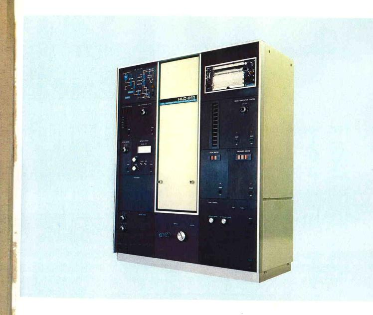
The TSK Model HLC 811 is a high temperature type gel permeation chromatograph with a total modular design. This model features a high speed analysis, variable temperature range from room temperature to 150°C, high sensitive detector, rotary syphon flow monitor, digital indication, and high performance. It just realizes the GPC equipment ideal.
