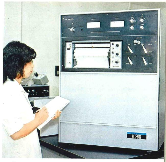
The Model **HIG:807** is a high performance liquid chromatograph designed specifically for preparative purpose. The system incorporates the many unique features developed by Toyo Soda that open up new possibilities for LC analysis in a number of fields. The adjacent chromatogram is an example of the 807's excellent performance.
