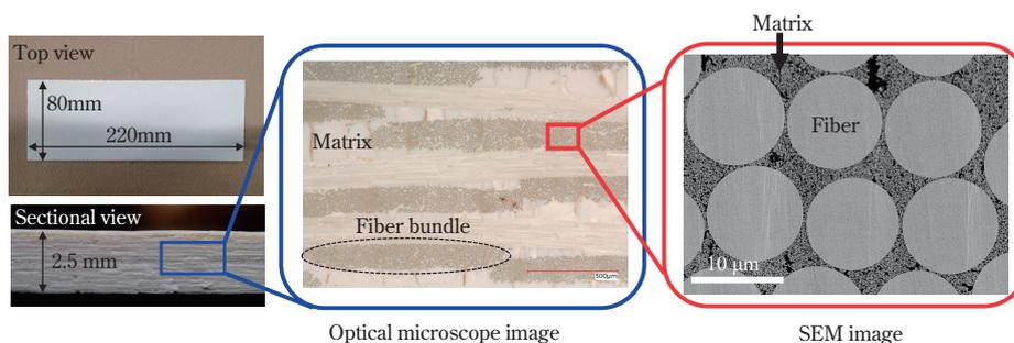
Fig. 3 Optical image and microstructure of TCM-02
