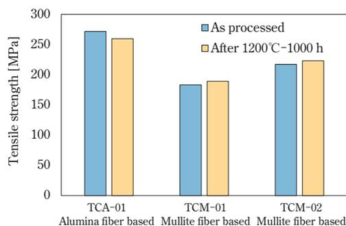
Fig. 4 Tensile strength of developed Ox/Ox as processed and after 1200°C for 1000h thermal exposure<sup>9</sup>
