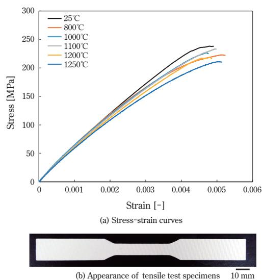
Fig. 5 (a) Stress-strain curves of TCM-02 and (b) appearance of tensile test specimen
