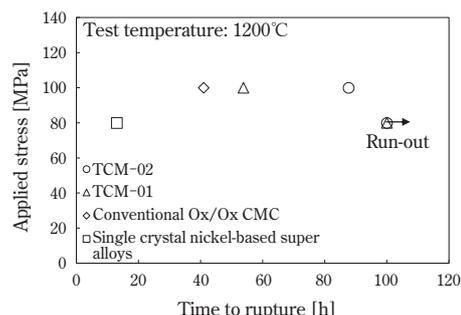
Fig. 9 Creep stress vs time to rupture at 1200°C
