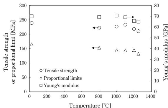
Fig. 6 Tensile properties of TCM-02 at different temperature
