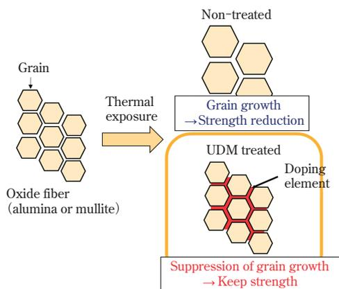
Fig. 2 Concept of uniform doping methods (UDM)<sup>10</sup>
