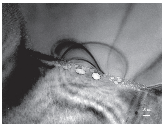
Fig. 9 TEM micrograph of residual pores at grain boundary in transparent zirconia ceramics.
