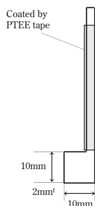
Fig 1 Geometry of the specimen used in electrochemical measurement
